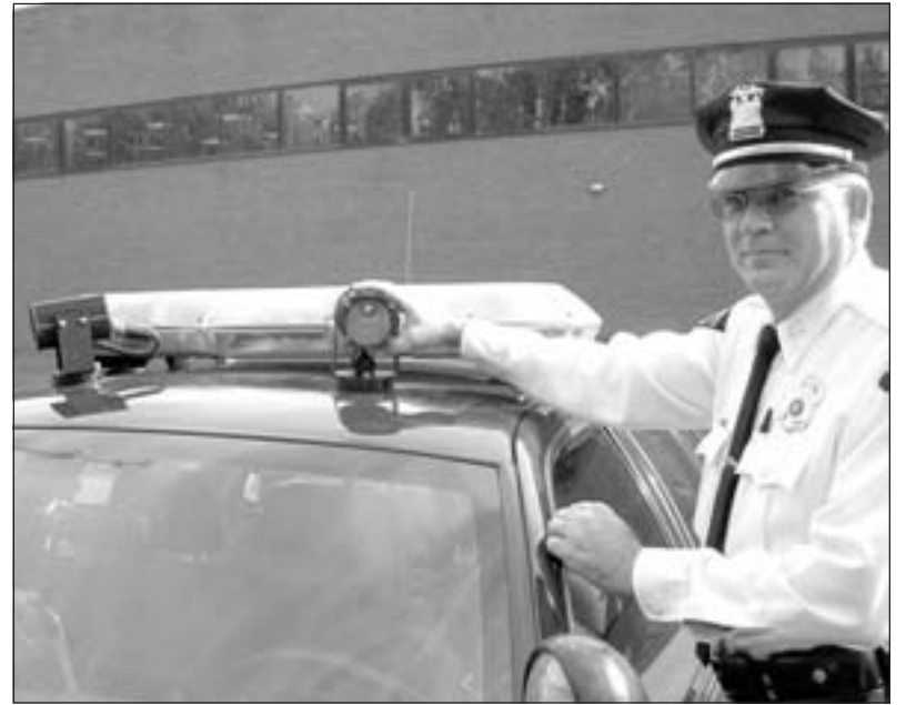
Captain Patrick McKenna adjusts the mobile plate reader that was recently installed on an Amherst Police patrol car. The device can read up to 1,500 license plates per minute.
